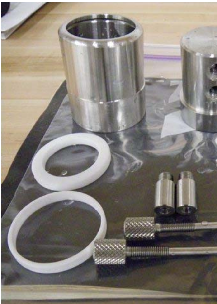
The well was constructed entirely of 316 surgical stainless steel, including this valve
