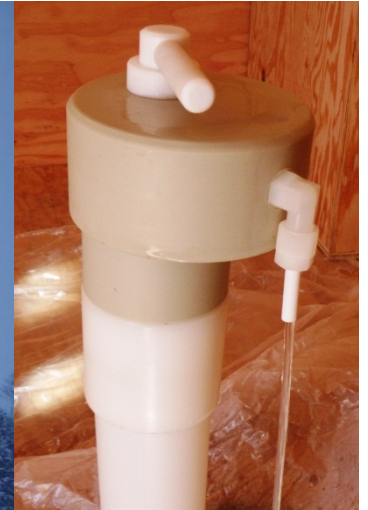
EGO-2 (Sept 2009) Acid-washed, high density polyethylene (Rotek, DK) well with polypropylene and Teflon valve
