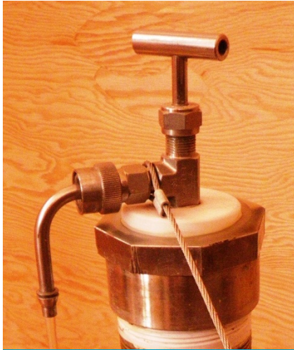
EGO-1 (May 2009) Surgical (316) stainless steel well and valve
