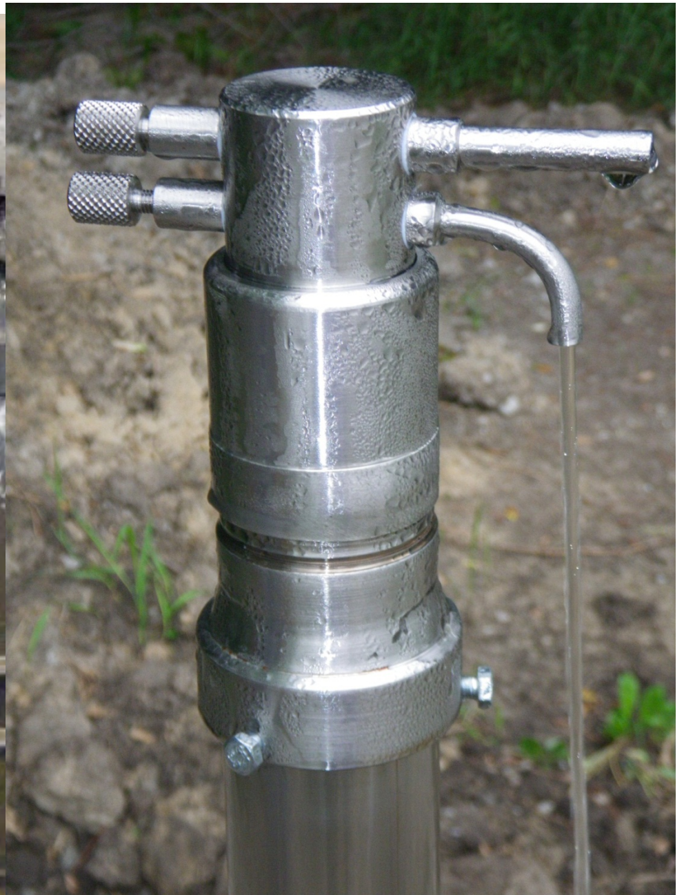
The well was constructed entirely of 316 surgical stainless steel, including this valve
